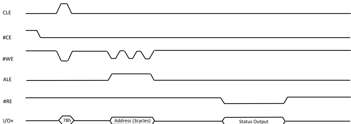
Figure 9-7 Read Status Enhanced (78h) Operation
